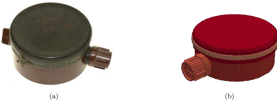
Figure 2.7: (a) The real PMN landmine (b) The numerical equivalent of the PMN landmine developed in [5].
