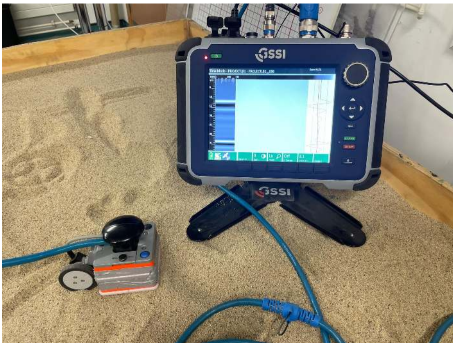
Figure 5.1: The GSSI 2GHz ‘palm’ antenna setup. This includes the antenna itself and the SIR system.
