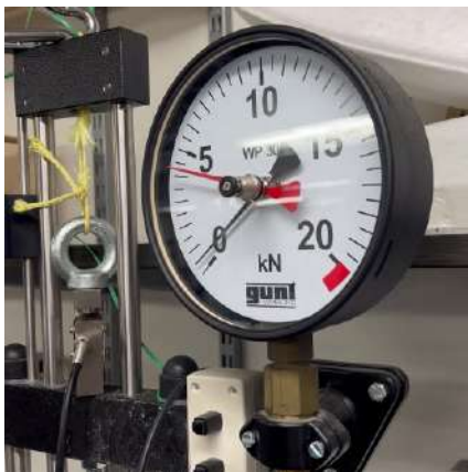
Figure 23: Loop specimen during fracture, red and black dial indicators show maximum and current load.
