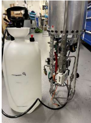
Figure 13: Filling tank with hand pump
