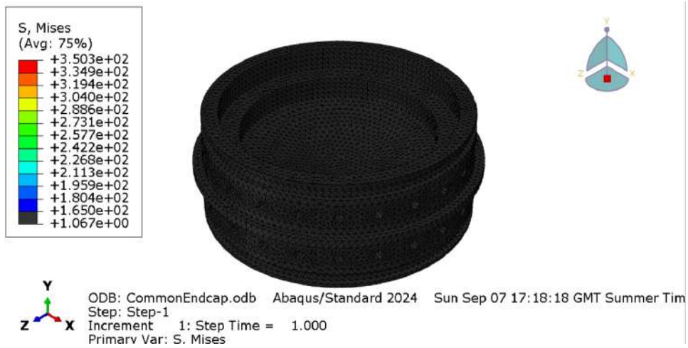
Figure 77: Common Bulkhead with Top Pressurized
